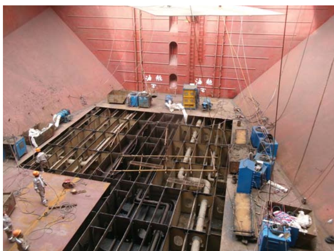
Steel renewal of cargo hold tank tops.
